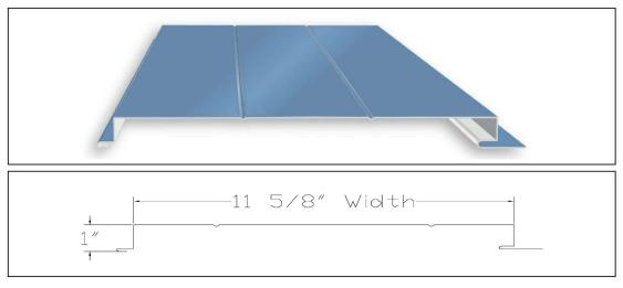
L- Panel is a maintenance free and economical panel for open spans. It can be used for various applications such as soffit, liner, fascia, and even ceilings. It is available in 23 stock colors as well as 8 premium colors, all of which are manufactured in 24 ga. panels. It can be configured as smooth, grooved, or perforated.
