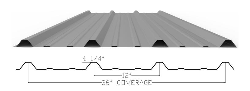
PBR Panel – A higher ribbed profile that is ideal for pre-engineered metal buildings. R-panels offer strength, attractive profile and long lasting performance. Manufactured in 26 ga., and available in 22 colors. Available in 24 ga. and 22 ga. by special order. Minimum recommended slope is 1:12 with sealant.
