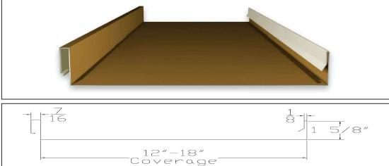
SL175 is an excellent structural standing seam roof panel that can be used in various roof, mansard, and fascia applications. Its design allows it to be applied to various solid substrates and even open purlins. This panel offers hidden clips and a snap-lock seam, which takes away the need for job site seaming. It is available in 32 PVDF colors in 24ga, and 19 WXL and 5 PVDF colors in 26 ga. The minimum recommended slope is 2:12 with sealant.
